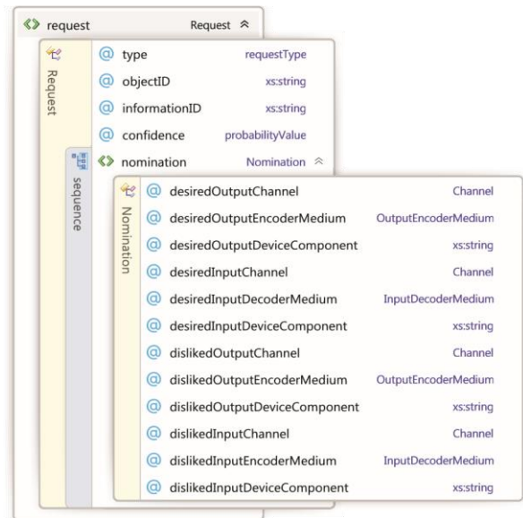
Figure 3. Visualization of the XML Schema definition for a request with nomination specification. It includes diverse attributes that are used to characterize the user’s demands on the UI configuration.
